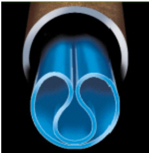
Shape of folded pipe during installation
